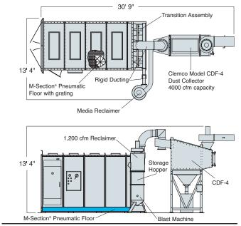
**M-Section**<sup>®</sup> **Pre-Assembled Blast Room** Recommended for fine glass bead and ALOX, or other lightweight media. Includes pneumatic recovery floor, and cyclone media reclaimer.
