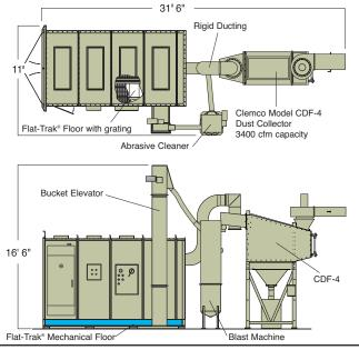
**Flat-Trak® Pre-Assembled Blast Room** Recommended for most recyclable media. Includes low-profile mechanical recovery floor, bucket elevator, and air-wash abrasive cleaner.
